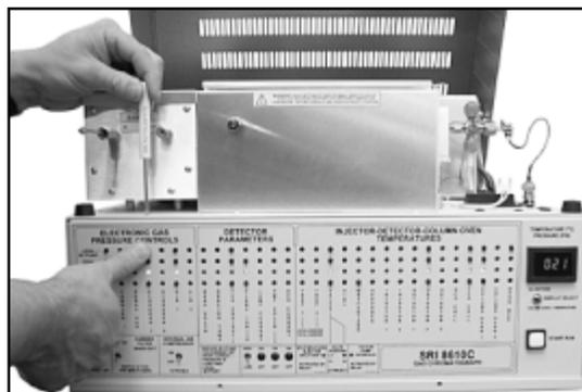
3. Set the NPD detector temperature to 250°C: hold down the SETPOINT button while turning the detector heat trimpot until the desired setpoint is visible in the LED display.
