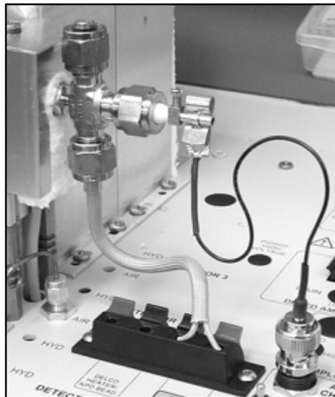
The NPD is similar in design to the FID, except it uses a thermionic NPD bead to generate ions in a hydrogen and air plasma. Like the FID, the NPD uses a stainless steel jet to deliver sample-laden carrier gas and hydrogen gas to the detector, and a positively charged collector electrode that also serves as the detector exhaust. The NPD bead is positioned between the jet and the collector electrode. The tip of the NPD jet is slightly different from that of the FID jet.
