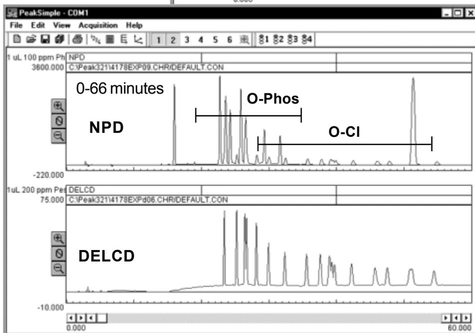
Sample: 1µL 100ppm Organophosphorus pesticide standard mix 8270 + 100ppm Organochlorine pesticide standard mix 8081
