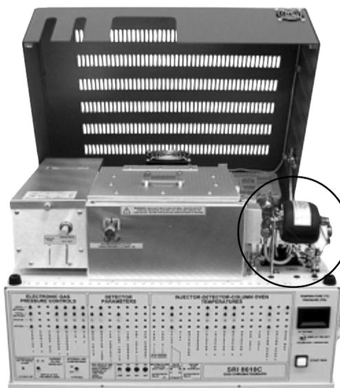
The NPD may be combined with the DELCD for pesticide screening. The NPD detects Organo-phosphate pesticides and the DELCD detects the chlorinated pesticides.
