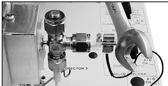
GC’s front control panel under the heading “DETECTOR PARAMETERS.” Verify that the FID flame is lit by holding the shiny side of a chromed wrench directly in front of the FID exhaust vent. The flame is lit when condensation is visible on the wrench surface.
