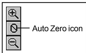
8. Zero the data system signal by clicking on the Auto Zero icon on the left side of the chromatogram window. Inject a sample containing ethane into the gas sampling valve through the sample inlet on the front of the valve oven. Start the run by pressing the computer keyboard spacebar, or by pressing the START button on the front of your GC. Note the elution time of ethane.
