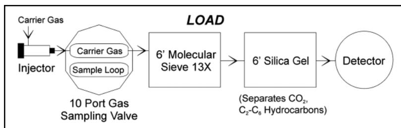
After the elution of the CO peak, the valve is switched back into the LOAD position, and the C<sub>2</sub>, CO<sub>2</sub>, and higher hydrocarbons come off the Silica Gel column.
