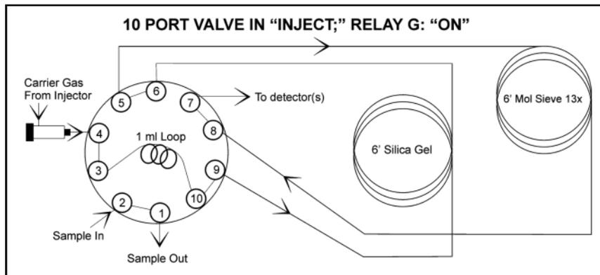
At the beginning of the chromatographic run, the valve is actuated to the INJECT position, depositing the sample loop contents into the carrier gas stream and directing it to the two analytical columns, which are connected in series through the 10-port valve.
