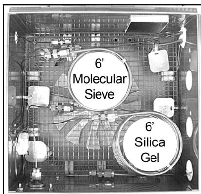
The MG#1 allows you obtain complete analyses of the fixed and natural gases listed above with a single injection. The MG#1 achieves this using a 10-port gas sampling valve with a 1mL sample loop in the heated valve oven, and two columns in the temperature programmable column oven.
