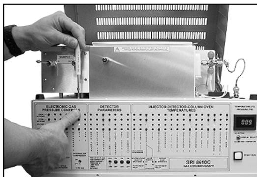
4. Set the valve oven temperature to 90°C. If present: set the FID/Methanizer temperature to 380°C; set the HID temperature to 200°C.
