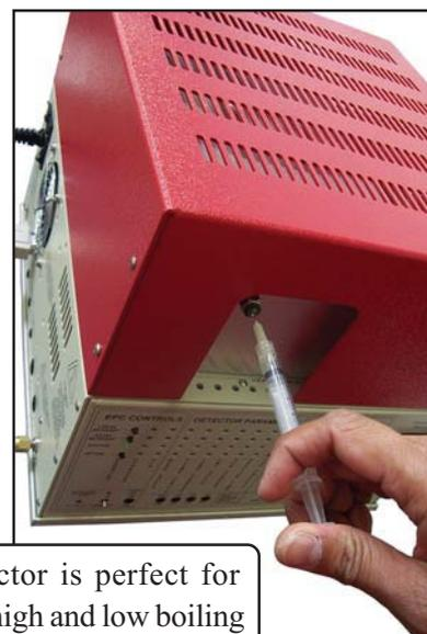
The On-Column Injector is perfect for liquids and gases with high and low boiling analytes. Even very high temperature analyses are easily performed using simple, reproducible on-column injection.
