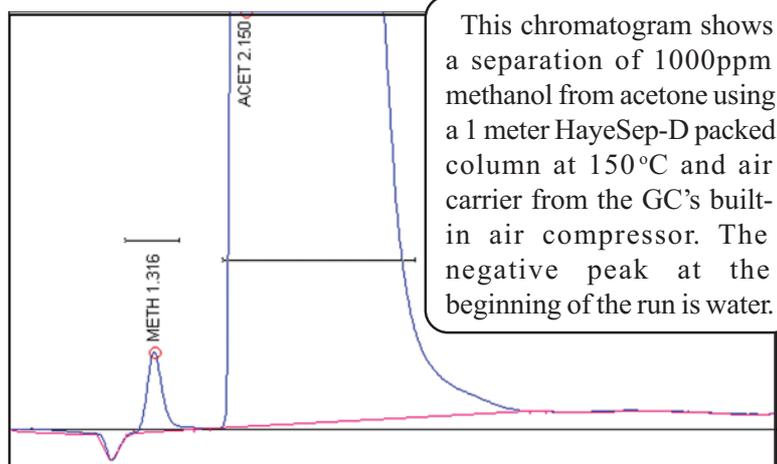
The CCD is about as sensitive as a TCD, but it has the hydrocarbon selectivity of an FID while capable of operating on air alone. Because the CCD needs no compressed gases like hydrogen or helium, it can be used in SRI's Gas-less™ GCs where a built-in, "whisper quiet" air compressor supplies the ambient air carrier gas.
