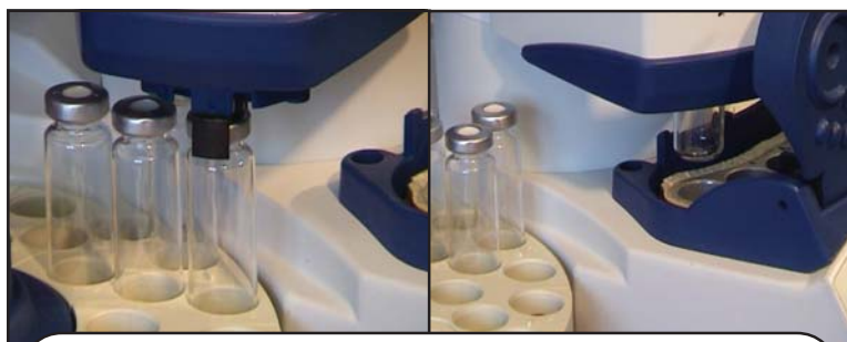
The HT200H picks up the vial and places it in the incubator
